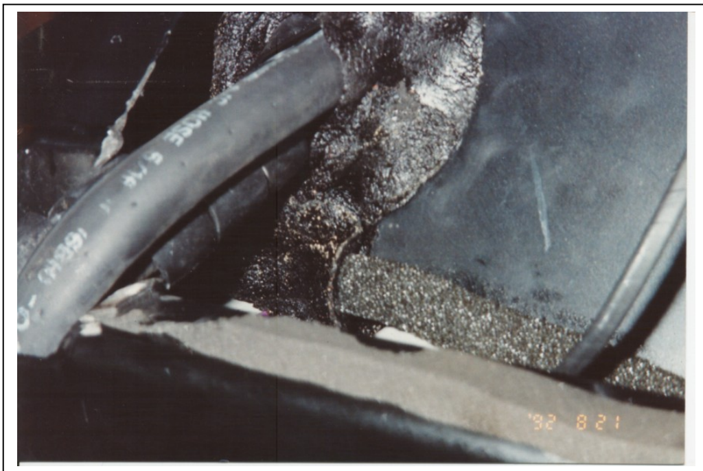
AC hoses notched and sealed through plastic shroud.
